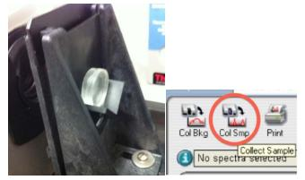
Place your sample in the FTIR. Click on the Collect Sample (Col Smp) button on the menu bar.
